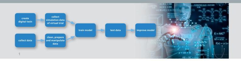
1 Hybrid machine learning workflow: experimental data is augmented with simulation-based data
