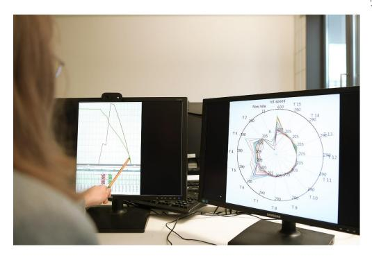
Julia Burr checks the results of the algorithm that suggests the settings for the extrusion machine. The left-hand screen shows the pressure and temperature curve of the melt in the extruder. The right-hand screen shows a Spyder plot with various suggested settings. © Fraunhofer ITWM
