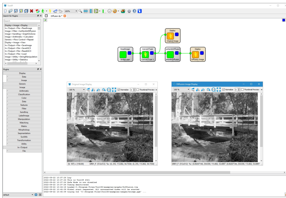
Figure 3.1: ToolIP with a minimalistic example graph.
