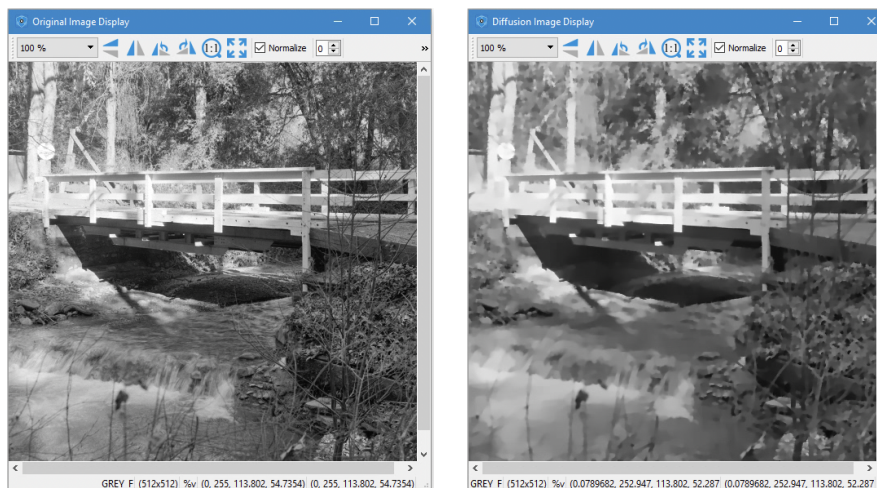
Figure 3.5: Effect of the morphological opening on the image BRIDGE.PGM.
